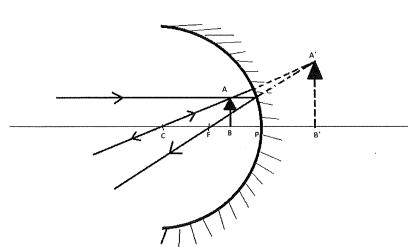
Ans: Nature of the image formed is virtual, erect and enlarged. The image is formed behind the mirror.
